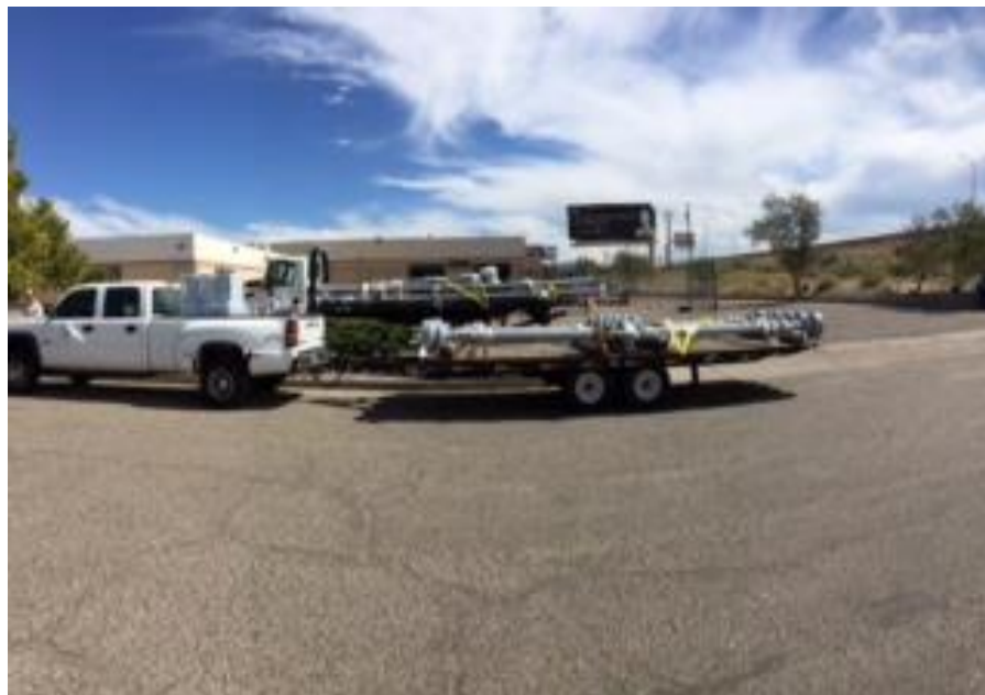
Traffic electricians picked up 28 light poles and associated hardware from a powder coating vendor in Albuquerque for the Central Avenue Phase 2 Project. Crews will reinstall the poles upon contractor completion of conduit installation and wiring.
