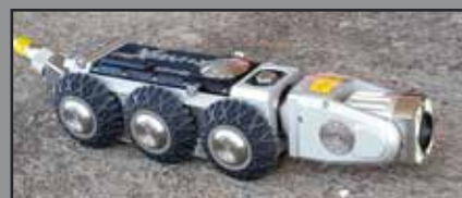
New sewer video camera equipment will permit crews to inspect inaccessible sewer lines.
