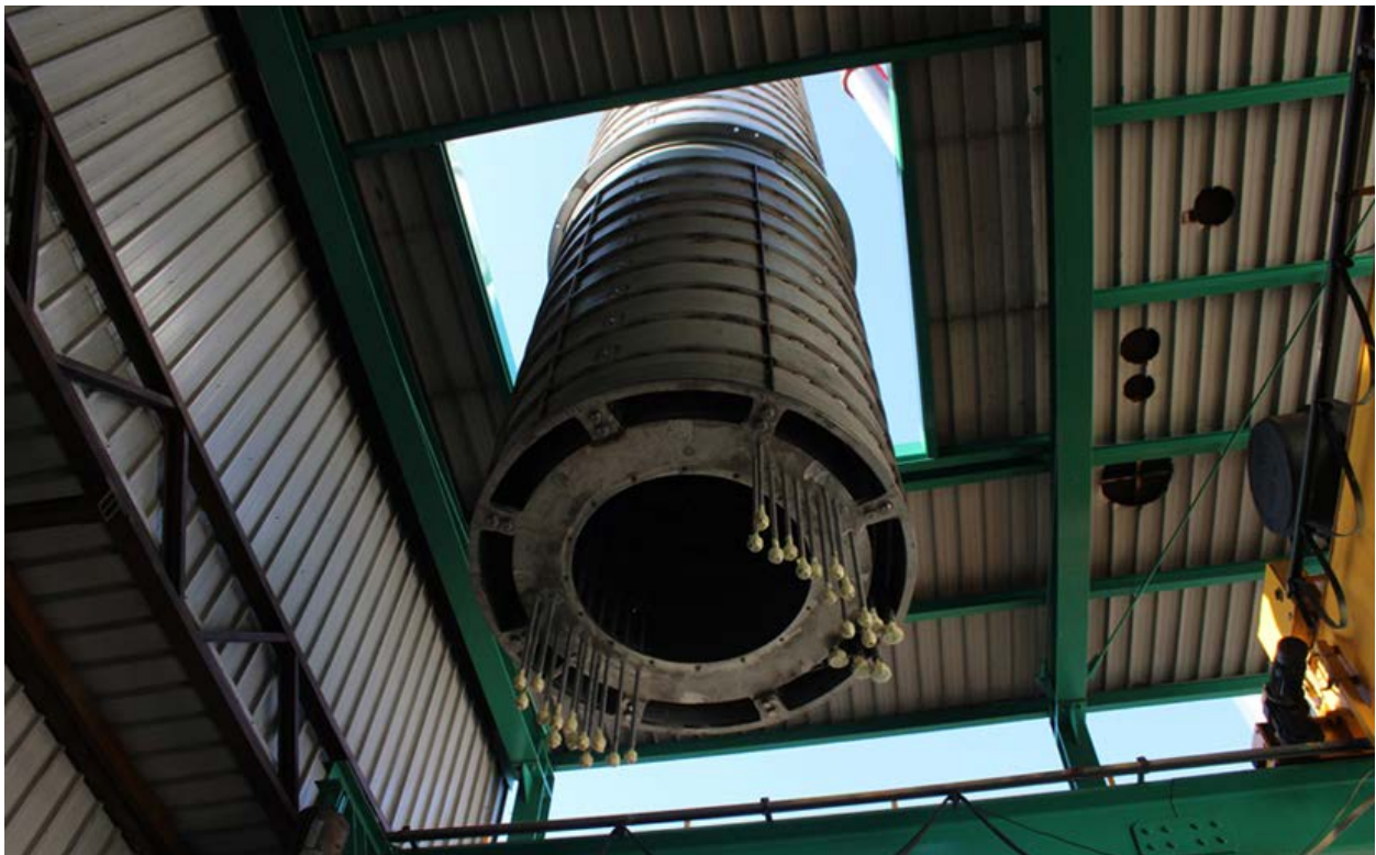
c. Helical Coil Steam Generator testing at SIET SpA in Piacenza, Italy
