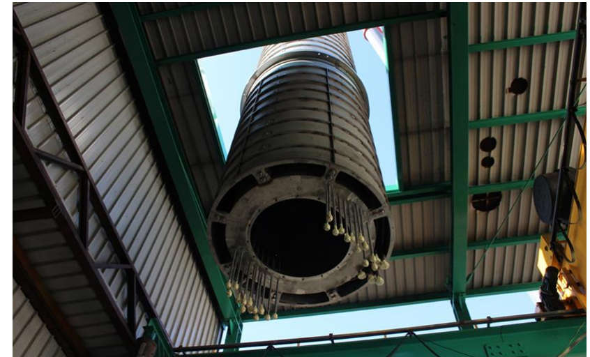
Helical Coil Steam Generator testing at SIET SpA in Piacenza, Italy
