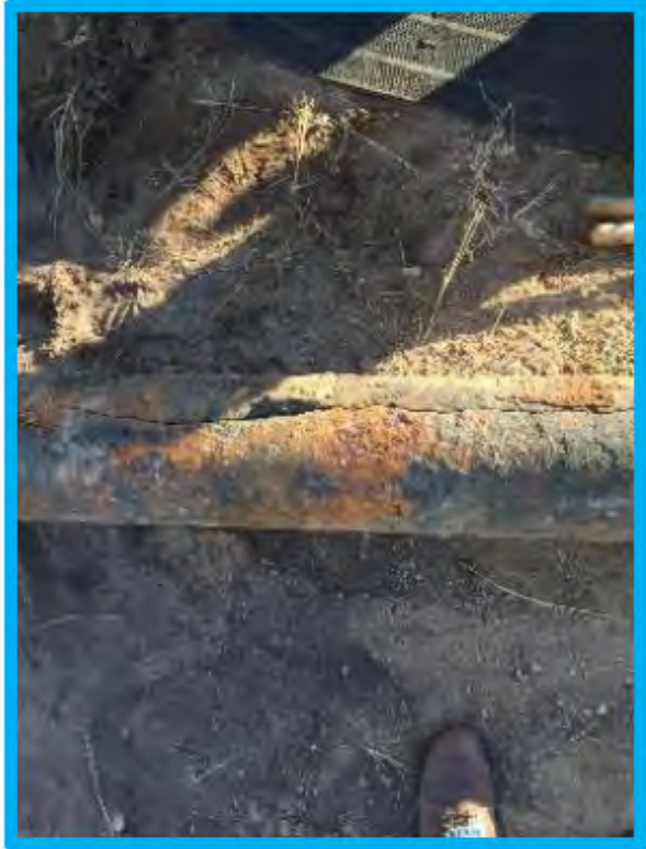
Split in Cast Iron Transmission Line
