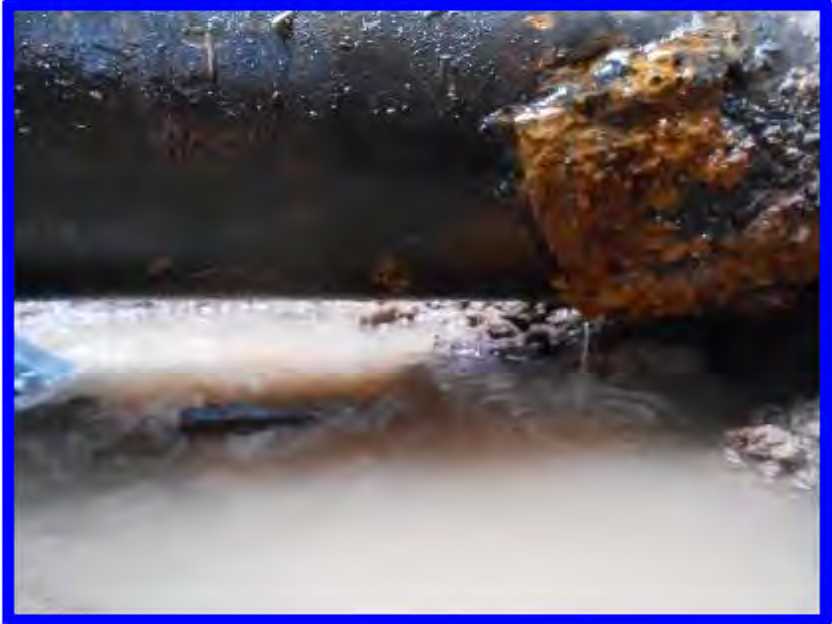
Corroded Cast Iron Pipe
