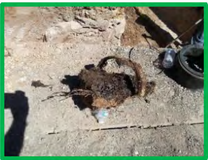
Root Ball Removed From Sewer Main
