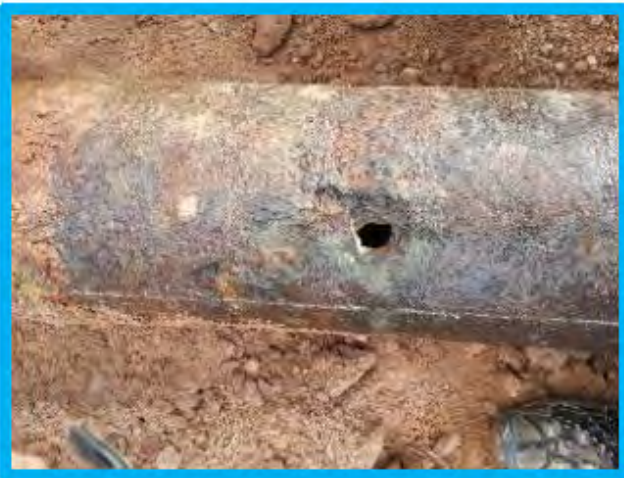
Corroded Cast Iron Pipe
