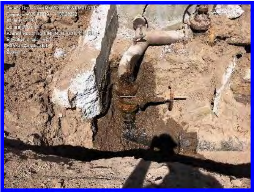
Corrosion Leak on Steel Pipe
