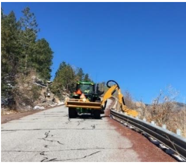
A crew member is seen clearing brush behind guard rails on Camp May Road with the boom new mower.
