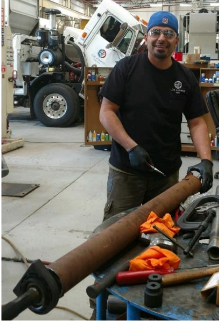
Raul Lujan, Fleet Mechanic II repairs a drive shaft.
