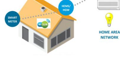
**TEPCO B-ROUTE:** Communication Between Smart Meters and HEMS HAN: Communication between HEMS controller and HAN device
