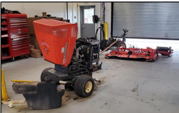
Robert disassembles a mower to diagnose a transmission issue; a fixed a broken spring and reassembled.
