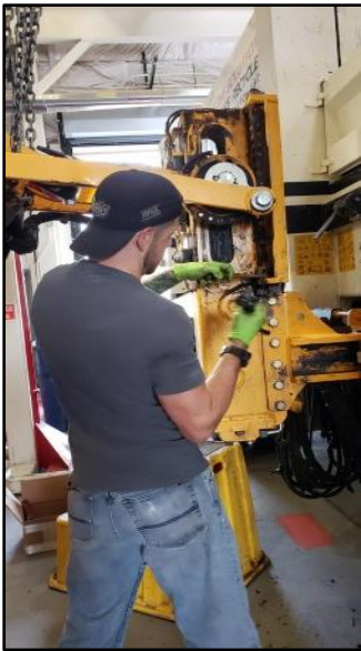
John replaces the dump chain on the Environmental Service's truck. These trucks service between 600 and 1000 roll carts a day depending on the route.
