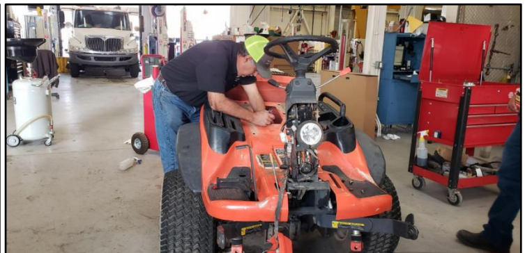
Robert disassembles a mower to diagnose a transmission issue; a fixed a broken spring and reassembled.
