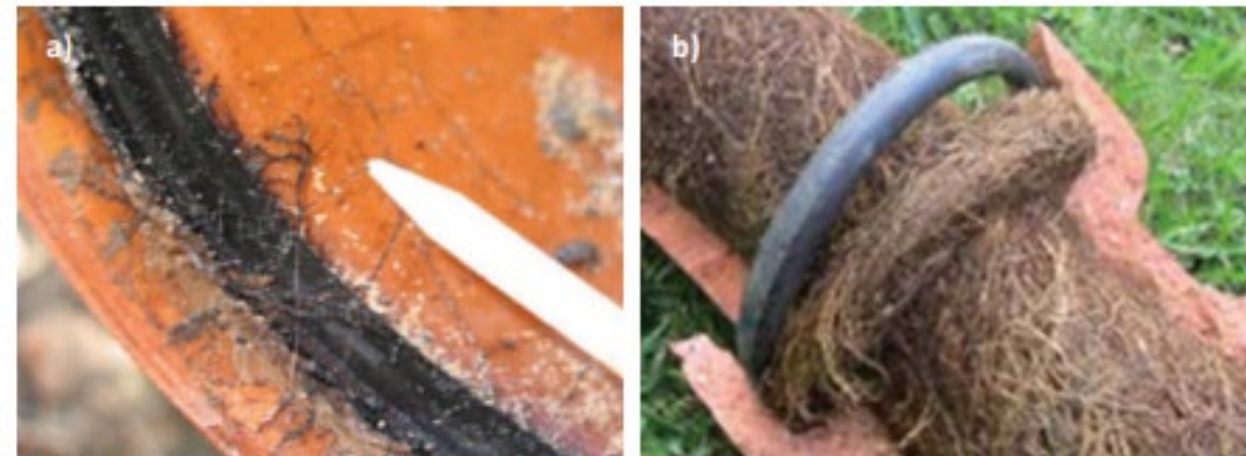
Figure 1. Roots in: a) modern PVC pipe [17]; b) old terracotta pipe – plugged pipe [18]
