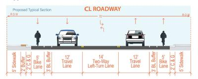
Includes: one 12-ft lane in each direction with a 14-ft twoway left-turn lane (TWLTL), 5-ft bike lanes, 5-ft sidewalk, and standard curb and gutter
