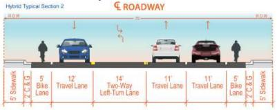
Includes: one lane in the westbound direction, and two lanes in the eastbound direction with a 12-14-ft two-way left-turn lane (TWLTL), bike lanes or multiuse path, 5-ft sidewalk, and standard curb and gutter
