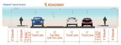
Includes: one lane in the westbound direction, and two lanes in the eastbound direction with a 12-ft two-way left-turn lane (TWLTL), 5-ft sidepath, 6-ft sidewalk, and standard curb and gutter
