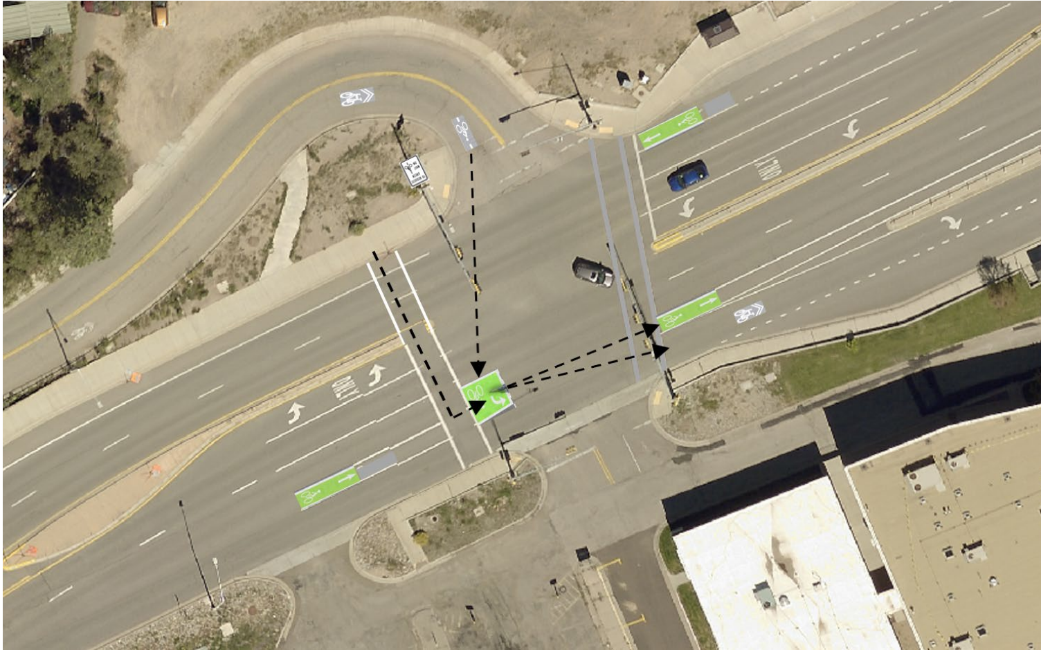
Diamond Dr/West Rd Intersection Conceptual Design for Bike Box Application
