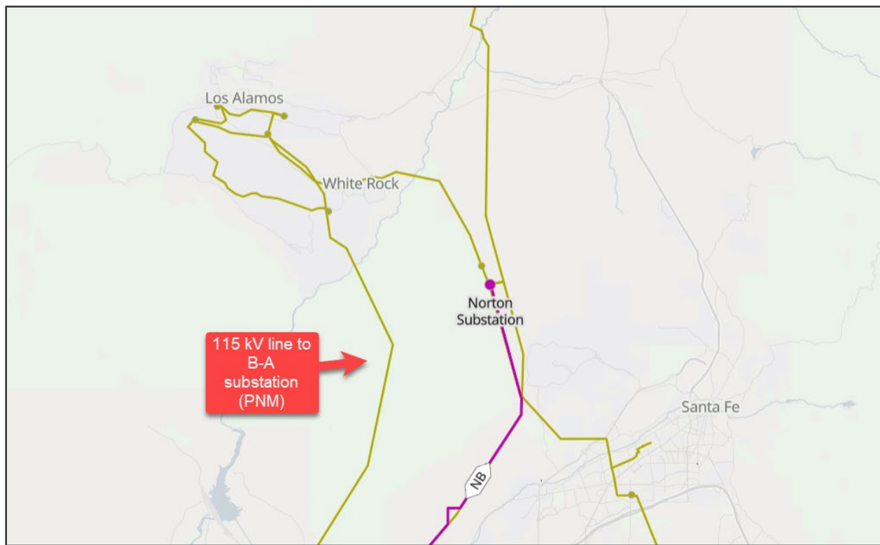
Figure 6-1: Transmission system of Los Alamos County 30
