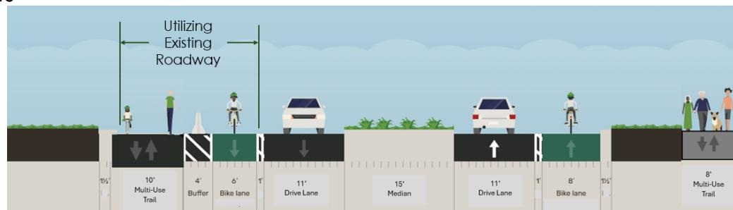
**RECOMMEND WB Lane Reduction and Trail Placement on NM4**
