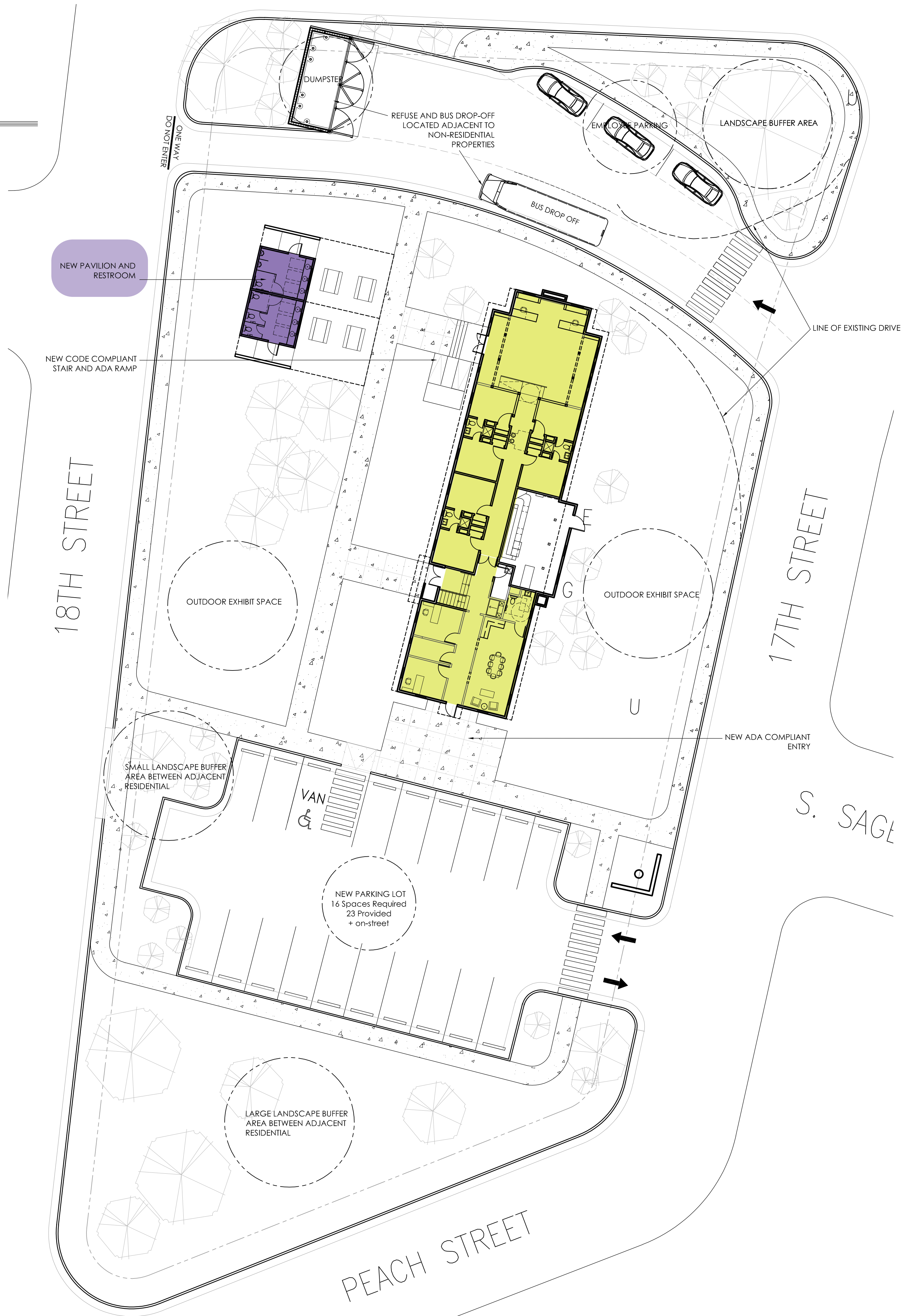
3 First Floor Site Renovation Plan Scale: 1/16"=1'-0"
