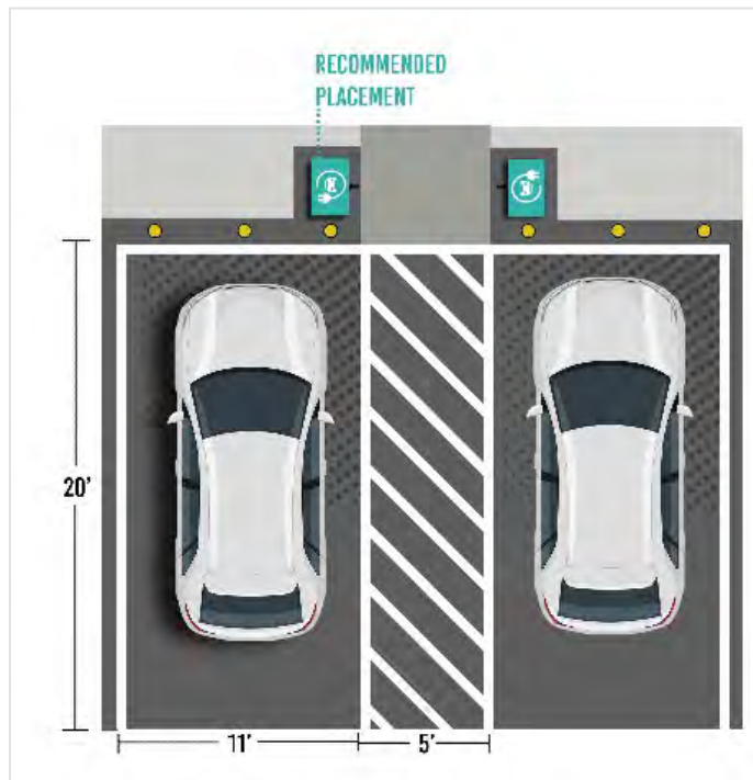
Figure 6-3: ADA Compliant EV Chargers in Parking Lot
