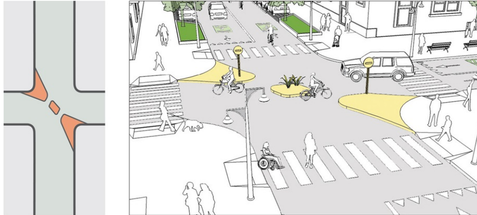
Figure 4.8: The modal filter allows pedestrians and cyclists to go straight through the intersection but cars must turn.
