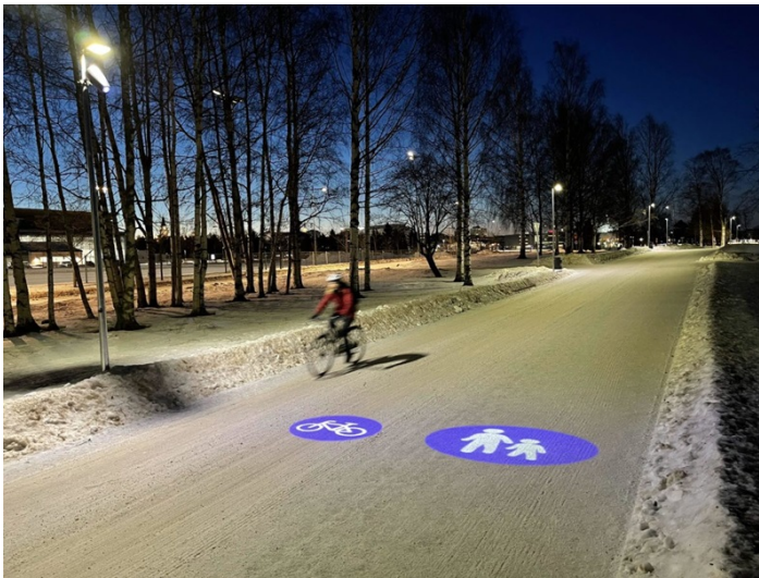
Figure 2.1: Cyclist on a bike path and walkway with lanes indicated by projected signs in Oulu, Finland
