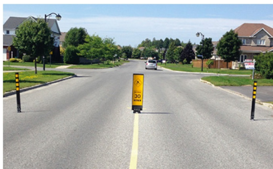
Figure 3.14: Side and center bollards on Kittiwake Drive, Ottawa, ON. These bollards reduced the 85% speed from 35 mph to 25mph without narrowing the road [8].
