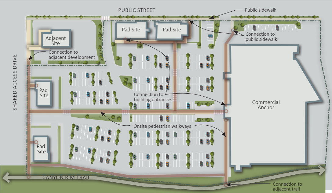
FIGURE 27: Required On-site Pedestrian Walkways
