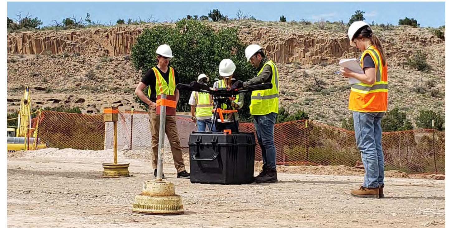
DPU's engineers coordinated a project with the UNM Civil Engineering program. Students are working on a process to use a drone to capture 3D LIDAR images of structural steel in reinforced concrete structures to perform quality assurance/quality control inspections. The project was conducted on the construction site of the White Rock Water Resource Reclamation Facility
