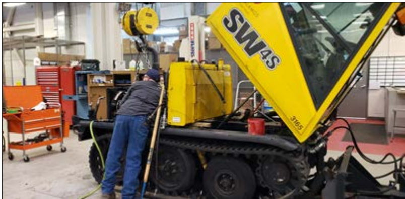
Leroy Campos seen here removing the engine to replace a leaking seal and then will have to reinstall the engine. This gives us an opportunity to get our snow removal equipment ready for the winter months.
