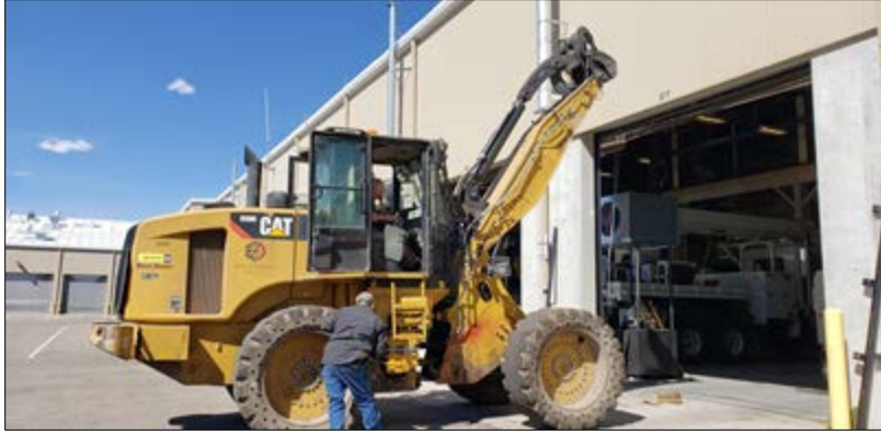
Matt and Leroy are performing hydraulic tests on the Eco Station front loader.
