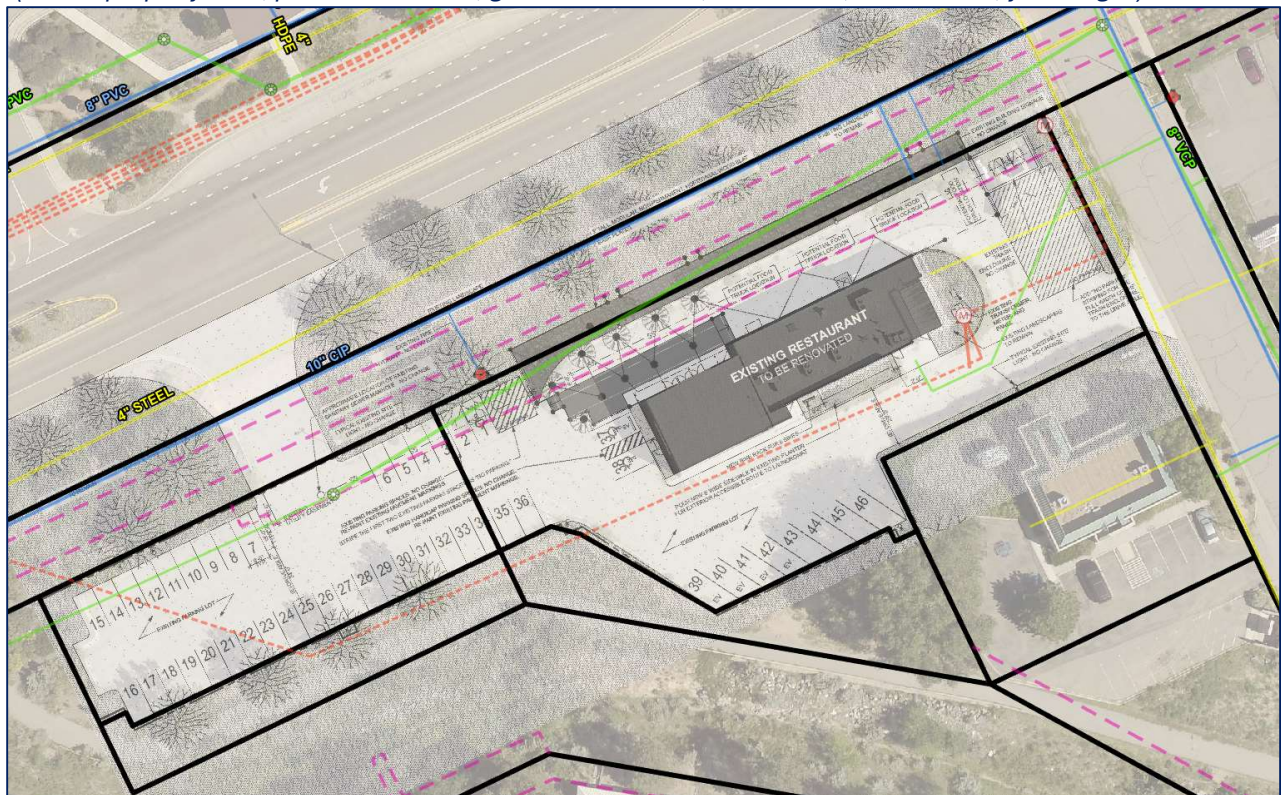
Figure 2: Proposed site plan aerial overlay with property lines, utilities, and easements. (black= property lines, pink = easements, green=wastewater, blue=water, red=electric, yellow=gas)
