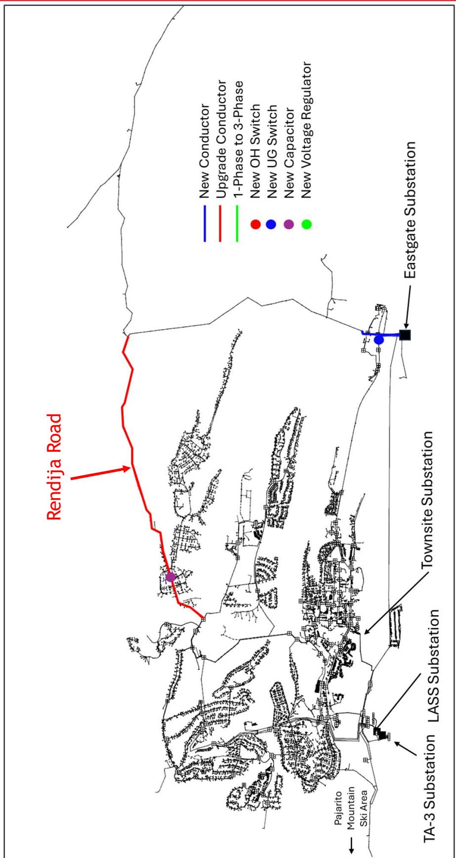
Upgrade approximately 3 miles of conductor to 477 ACSR to create a strong tie path from the Eastgate Substation to the north region of the service territory for normal load service and contingency support.
